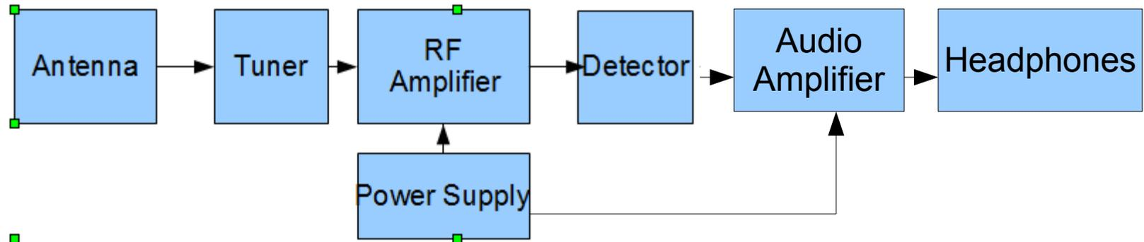
With this radio we have added an **amplifier for the audio** so it's louder. The Radio Frequency Amplifier was used to increase the power of the Radio signal. The Audio amplifier increased the volume in the headphones
