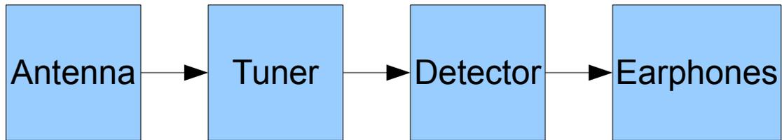
A block diagram may contain parts that are **not** inside the radio itself if that is self evident. Everyone knows that **earphones** are separate, and with such a simple radio as this an outdoor **antenna** is also separate.
