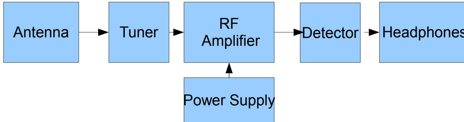
The antenna takes a weak signal (Radio Wave) and sends it to the tuner as a electrical signal. The tuner acts like a **filter** to separate the wanted radio signal from all the others. The **Radio Frequency Amplifier** causes the steady powerful current from the power supply to vary like the input signal. The **detector** extracts the **audio** information from the **carrier** and passes that to the headphones,
