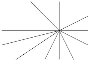
In this drawing think of the wave motion as straight out of the paper at the centre point. Thus all the lines are right angles to the wave's travel, and represent the direction of field 'vibration' or 'waving'.
