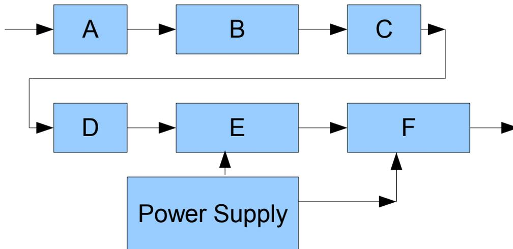
Boxes A, B, C, and D contain only passive circuits because they have no arrow coming from the power supply.
