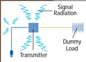
If you still have interference while transmitting into the dummy load, the source of the unwanted signal is definitely the cabinet or the power line. Proper shielding and grounding may solve a problem in the cabinet. If the problem is in the power line, a power line filter should be installed. Various types of power line filters are available from radio supply shops and electrical parts distributors. The diagram at left shows how to construct your own filter.
