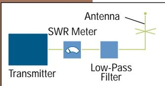
If the low-pass filter reduces the interference, then the cause is harmonic radiation. Adjusting the transmitter's internal circuits may reduce the unwanted signals. You may need to call an experienced technician to make these adjustments.
