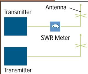
Test the equipment with no auxiliary RF devices installed. Test again as each device is installed. This method will help you find the exact source of the interference. If any device is the cause of the problem, try grounding it or remove it permanently.
